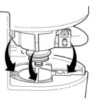
2. Once aligned, seat the sealant canister by lightly pushing down until you hear an audible click.
